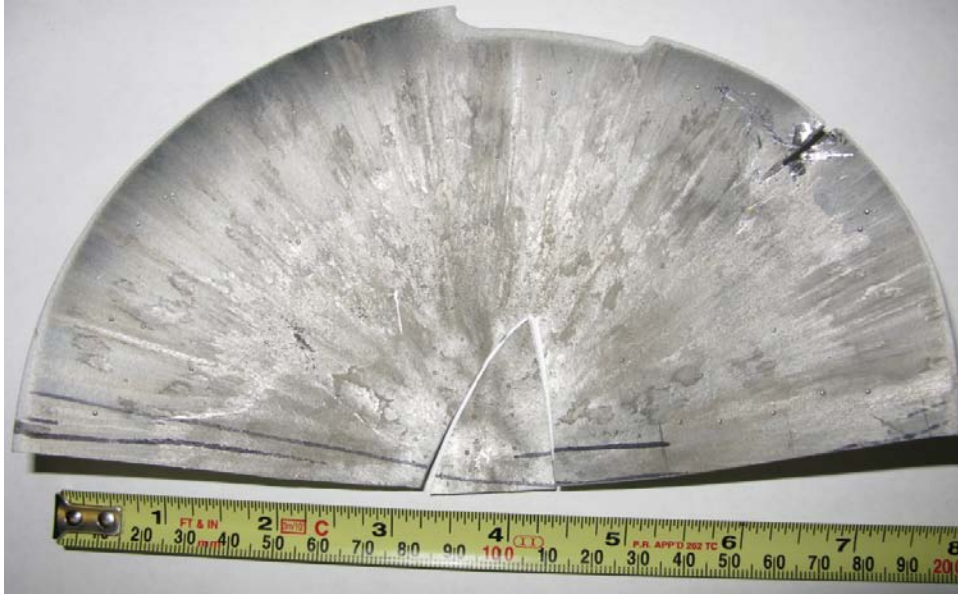
Figure 2. Triangular sample examined from the not- ruptured panel, in relation to the blast area
