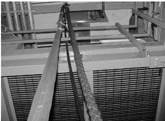
Radially compressive rope hanging next to a standard climbing rope.
