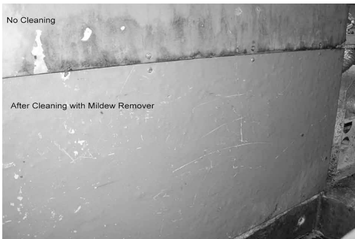
Mildew Growth Before and After Cleaning with Mildew Remover Inside T-39 Aircraft.
