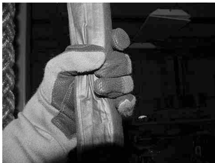
Squeezing by hand compresses rope minimizing need of friction.
