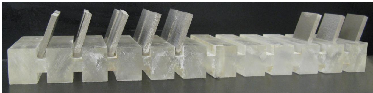
Figure 4. Corrosion rack configuration used for neutral salt fog and GM 9540P exposures.
