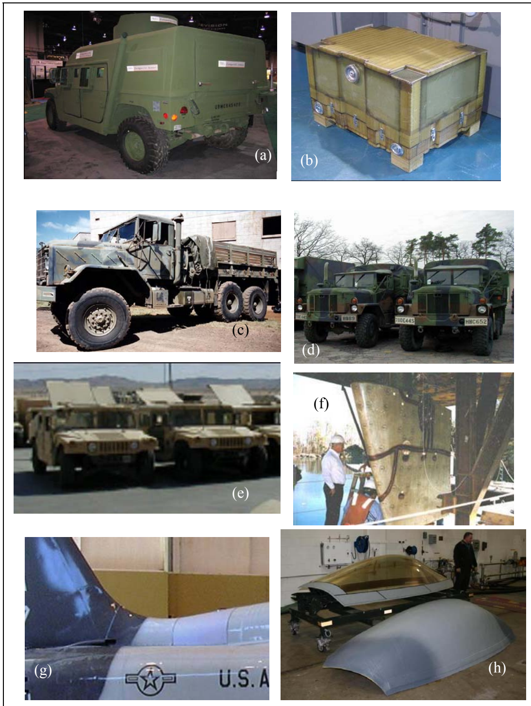
Figure 2. This program demonstrated/validated low-HAP VE resin composites for (a) HMMWV ballistic hardtop, (b) HMMWV transmission container, and one to two types of composite replacement hoods including (c) M939, (d) M35A3, or (e) HMMWV, and (f) MCM rudder, (g) T-38 dorsal cover, and (h) F-22 canopy cover.
