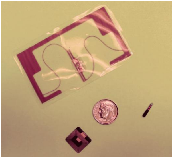
Figure 3.6: From [33], three different RFID tags and their relative size with an everyday object.
