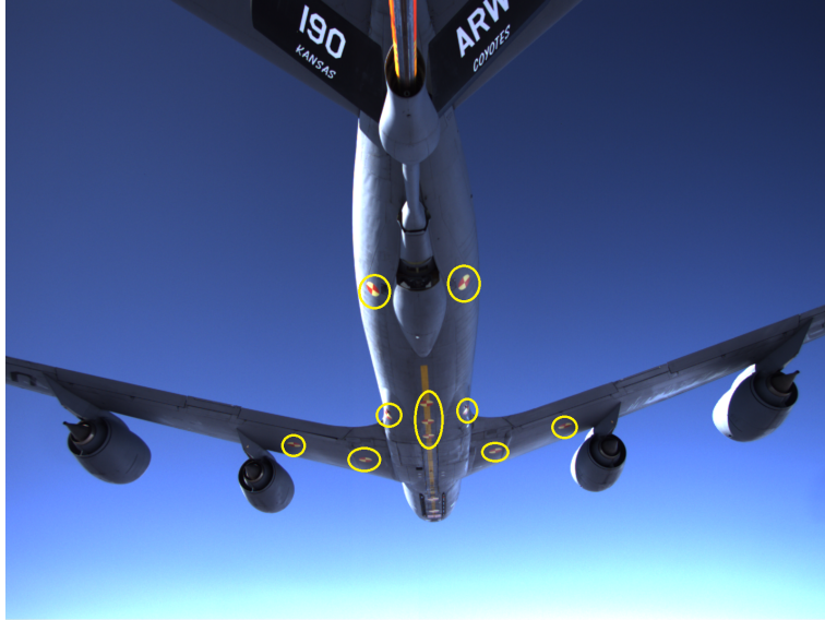
Figure 4.6: KC-135 with markers installed on the body of the aircraft. Markers have been circled with yellow. Picture taken in flight by Proscillica camera.
