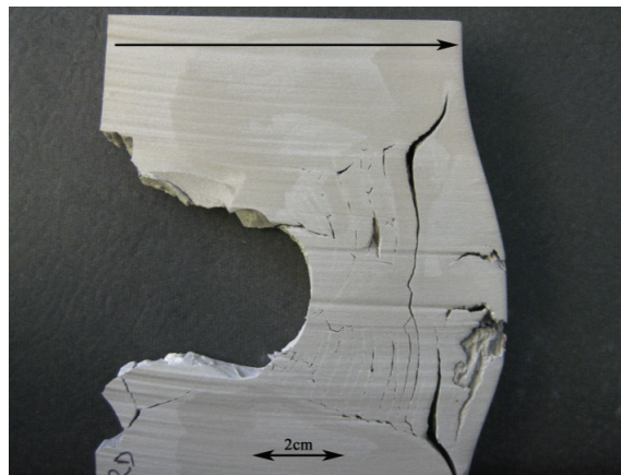
Figure 1. C-Partial sample, after cross sectioning, arrow indicates direction of impact.
