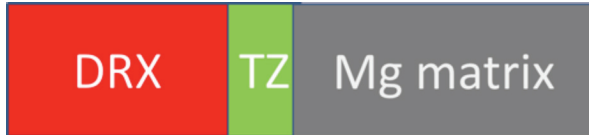
Figure 15. Diagram of shear band, and neighboring microstructure.
