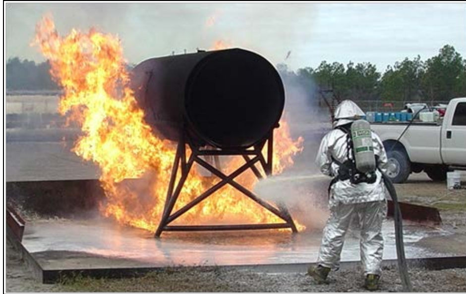
Figure 5. Firebane 1179 being applied to the engine protocol pool fire
