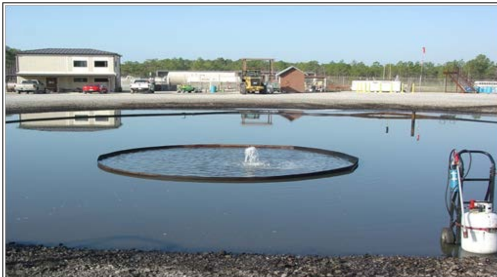
Figure 3. The 15-ft diameter pool fire ring being filled with JP-8
