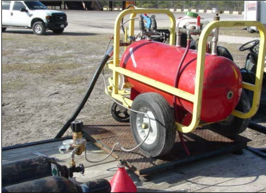
Figure 2. Modified Tri-Max 30 extinguisher positioned on scale
