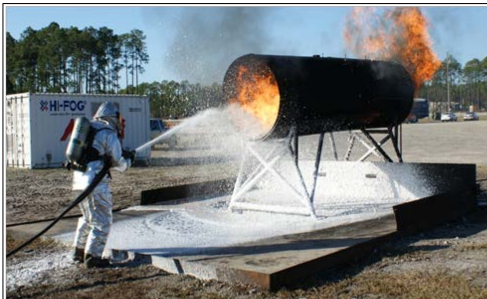
Figure 7. 50-percent Firebane 1115 foam blanket during engine nacelle test
