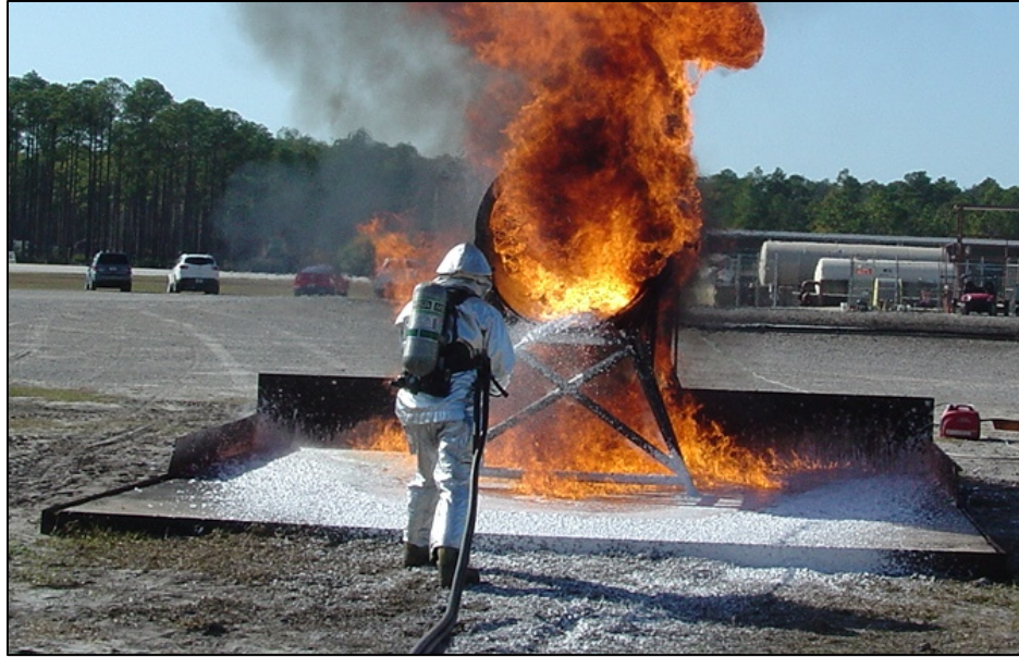
Figure 6. Firebane 1115 foam blanket during engine nacelle test
