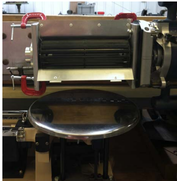
Figure 16. Tri-beam balance below CFF outlet
