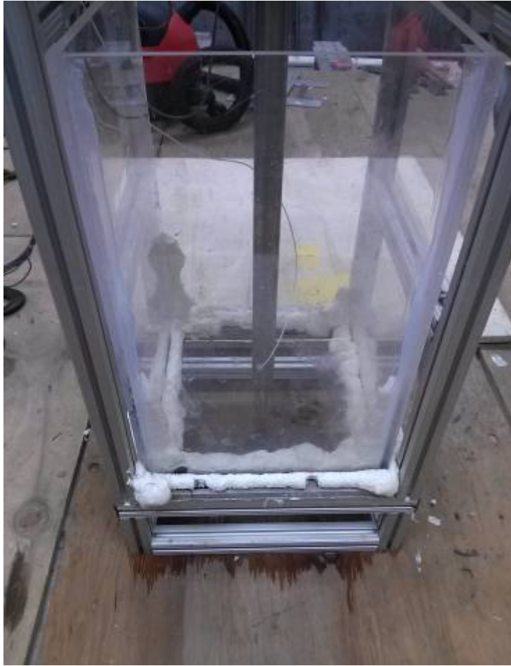
Figure 13. New setup using expanding spray foam as a second layer of water proofing.
