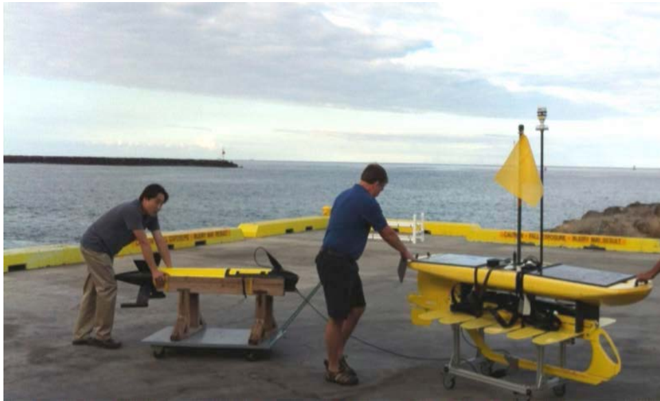
Figure 6. The Wave Glider and the tow body used in the dual-frequency echosounder experiment off the coast of Hawaii.
