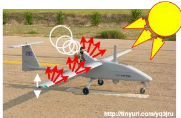
Figure 1: Ambient energy available on a UAV, including light, heat, and vibration
