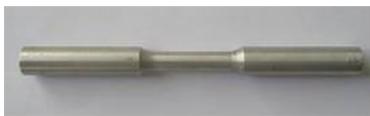
Fig. 2.2. Photo of round fatigue specimen
