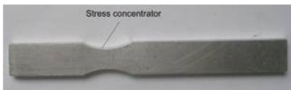
Fig. 2.4. Photo of flat specimens for corrosion fatigue tests.
