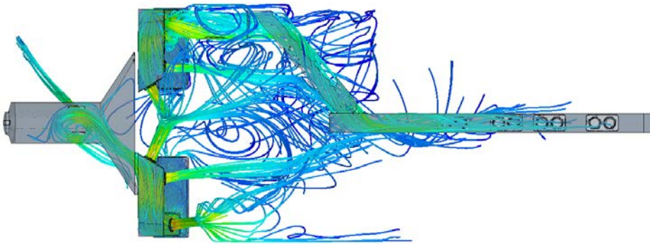
HVAC Duct Design/ Cooldown Sizing
