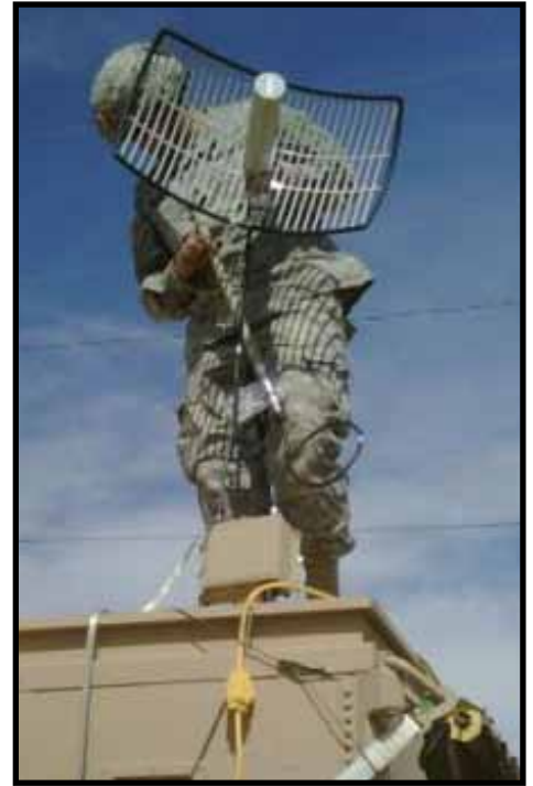
SASMO Soldier orienting a directional grid antenna for a Combat Service Support Automated Information System.
