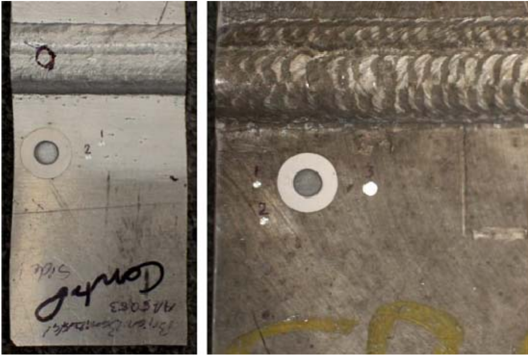
Figure 30. Locations for measurements for depth profile on both samples.
