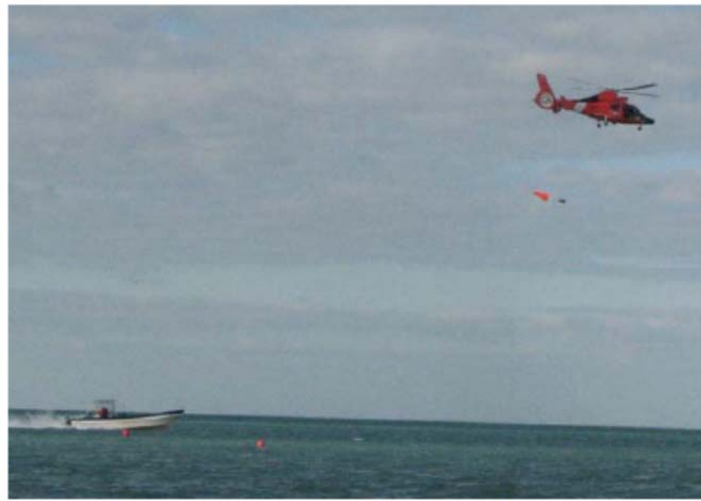
Figure 15. Deploying of Boat Trap from Coast Guard Helicopter (From [41])
