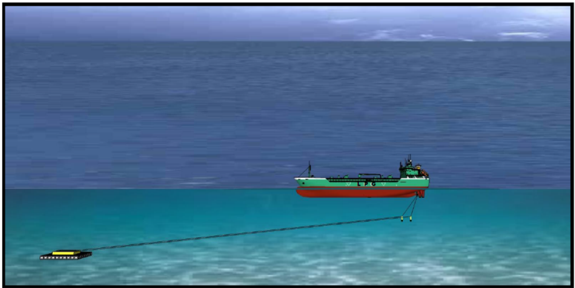
Figure 76. The UUVs launch the nets, are released from the ropes and retreat from the propeller. The ropes are about to wrap around the propeller and its hub.
