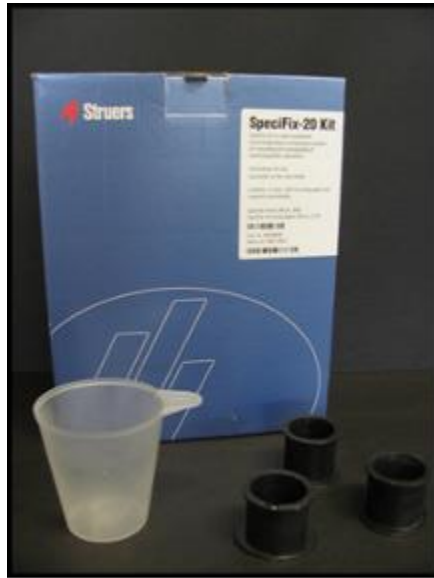
Figure 15. The Struers Specifix 20 mounting epoxy kit used to create composites with the carbon nanofibers and tungsten disulfide spheres. Also depicted are the cups used to mix the epoxy prior to pouring and the one and one quarter inch diameter molds used for curing the samples.
