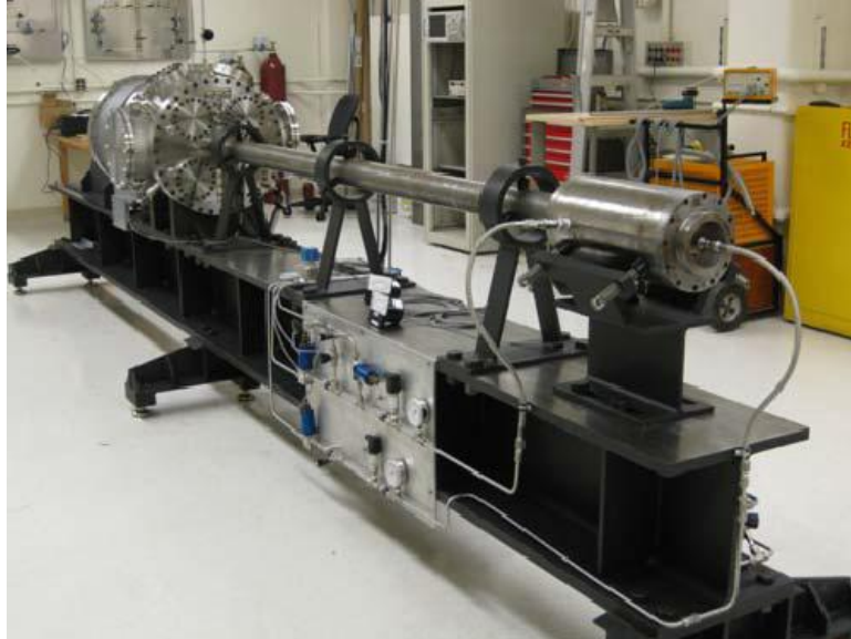
Figure 22. A picture of the gas gun setup. The breech is smaller cylinder on the right and the sample holder is the larger vessel on the left side of the barrel. From [26].
