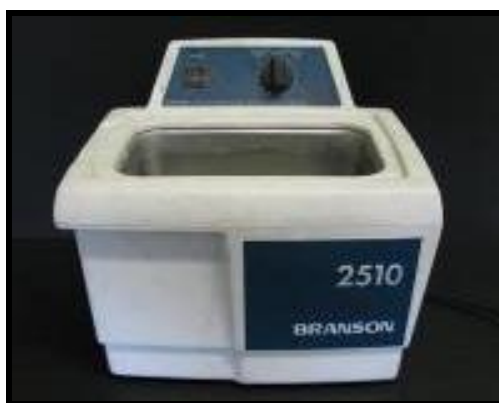
Figure 11. The Branson Ultrasonic Corporation Model 2510R-MTH Sonicator utilized to sonicate the tungsten oxide precursor and nickel nanoparticle catalyst.
