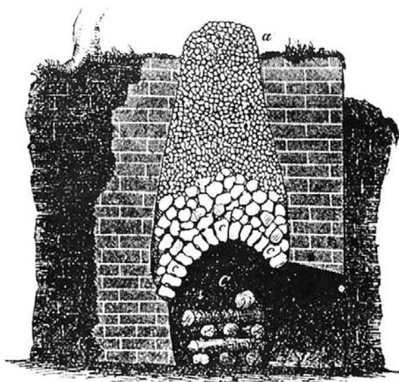
Figure 16. Cross-section of the base of an early wood-fired lime kiln (Gilmore 1874).
