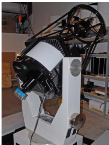
51 cm dia. Telescope for Placement in Chile
