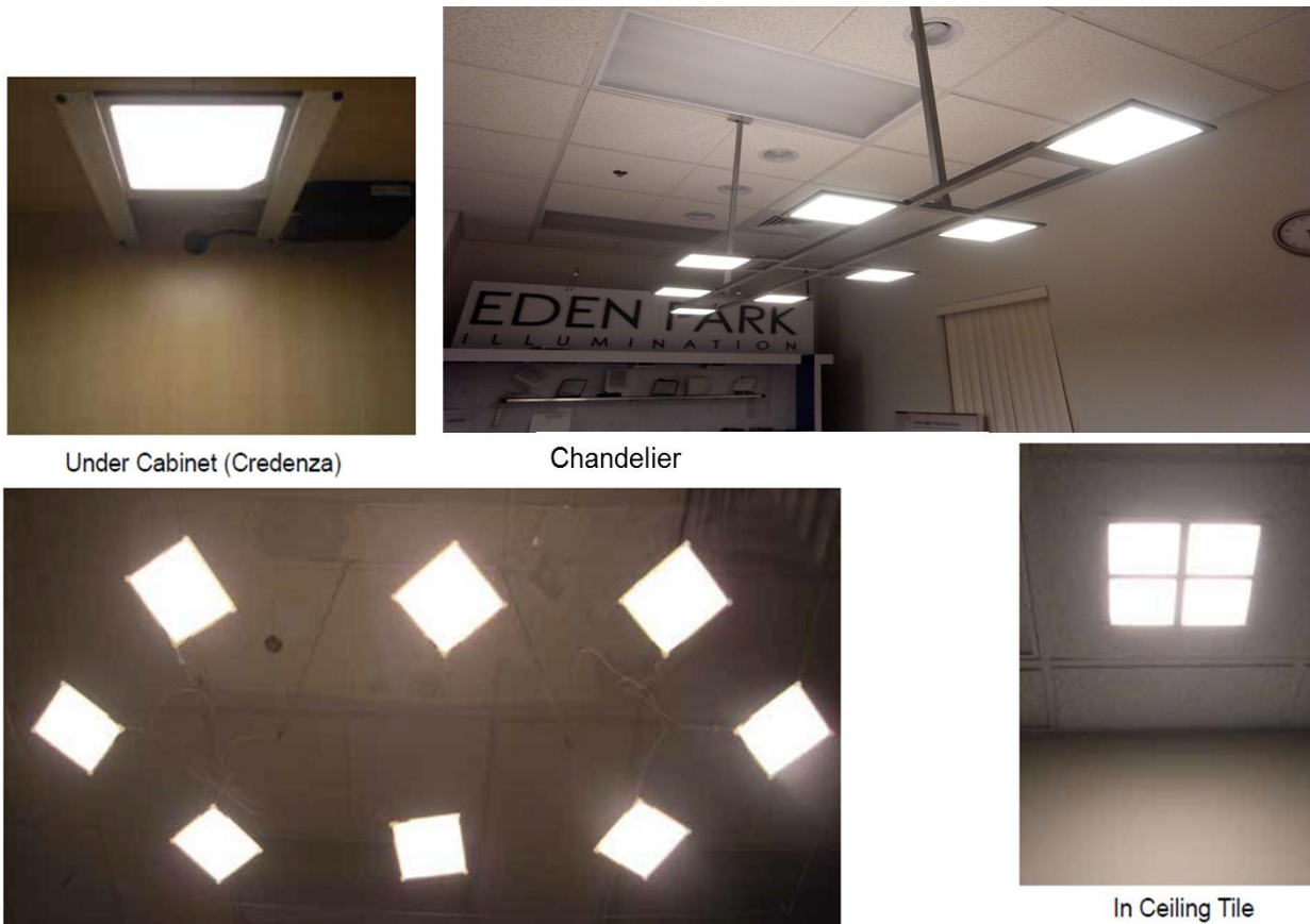
Fig. 12. Photographs of microplasma tiles which demonstrate their potential and versatile uses as a new lighting technology.
