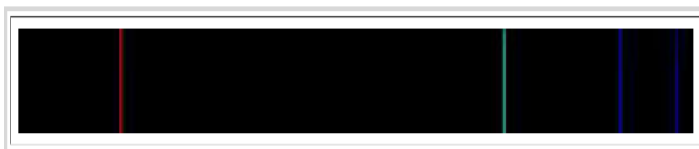
Figure 3. Hydrogen line spectra. From [7].
