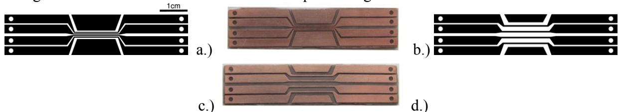
Figure 14. Toner Masks for Etching and Photographs of the Etched Chips
