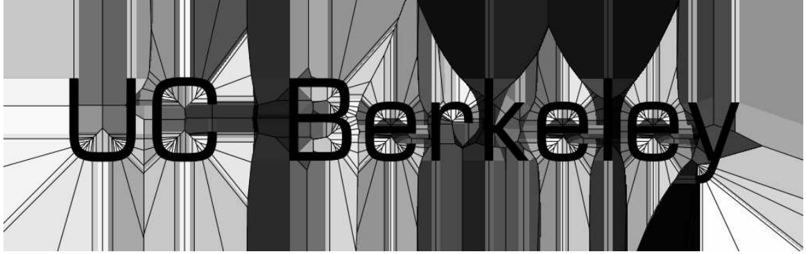
Figure 3: Fast distancing to piecewise-polynomial curves: the background shading from white to black indicates regions where the algorithm requires 1 to 5 elementary distancing operations respectively.
