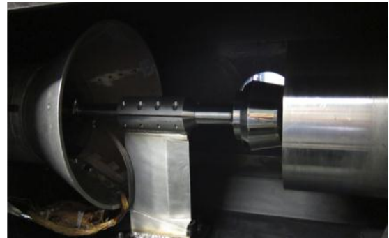
Figure 11: NASA Langley 93-10 flared cone model, on bench (left) and installed in M6QT (right)
