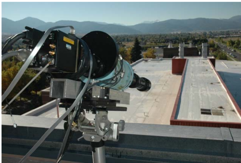
Fig. 5. Photograph of the API fitted with the telephoto front optics module to measure the polarization signature of smooth and rough metal plates under variable cloud conditions.
