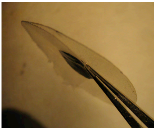
Figure 31. Figure showing separation of nanolatex films photothermally bonded together by intervening patch of SWCNT/nanolatex film after photoirradiation.
