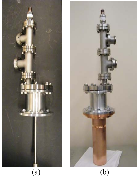
Fig. 4a,b Illustration of a beam management device a) without and b) with the anode present.
