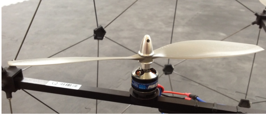
Figure 5: Motor, Propellor, and Speed Controller.
