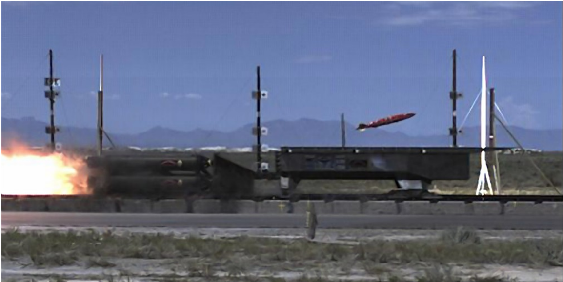
Figure 5. HIFEX sled testing demonstrating successful release.
