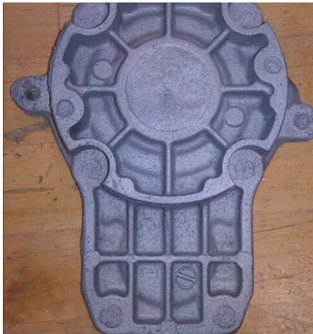
Figure 16: Casted part post sprue removal and sand blasting
