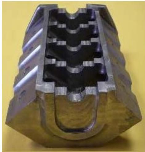
Figure 30. Engine block machined using CNC-RP to verify the design and generate process plan. Block is cast iron.
