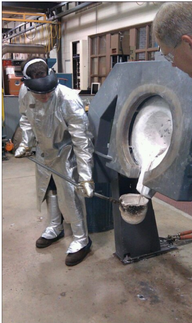
Figure 12: Zach Wilkoski and Randy Wells, lab technician, pouring Aluminum 356 at 1400 degrees F
