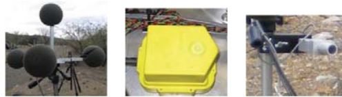
Fig. 1. Four acoustic sensors (top left), seismic sensor (top right) and passive infrared (PIR) sensor (bottom).
