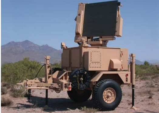
The air-defense radar for the Rapid Avenger missile system automatically detects tracks, identifies, classifies, and reports airborne threats. (Thales/Raytheon photo)
