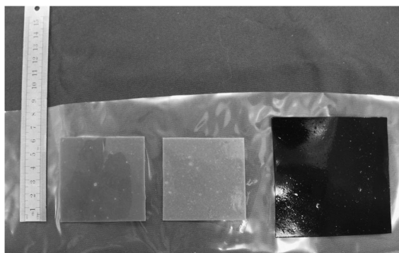
Figure 1. Adhesive specimens conditioned in (left) water at 70°C, (center) hydraulic fluid at room temperature, (right) hydraulic fluid at 70°C. The specimens on the left and at the center have approximate size equal to 60 mm (the initial/nominal size is 60 mm).
