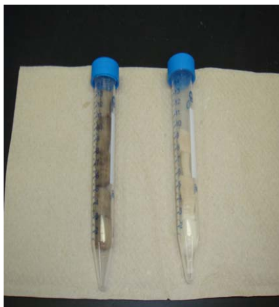
Figure 5: Unprocessed Potatoes (Left) and Potatoes 12 h after Processing at 4350 psi for 45 min (Right).
