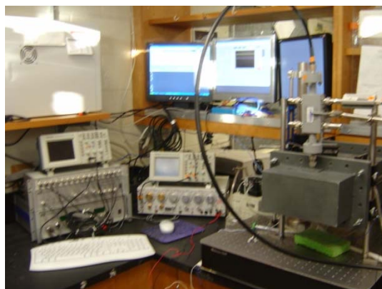
Figure 5. Photograph of the waveguide-based exposure system that was used for assessing RF effects on skeletal muscle contraction
