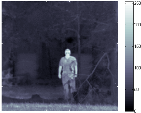
Figure 9: A MWIR thermal image mapped to 256 bins with values in [0\ 1]
