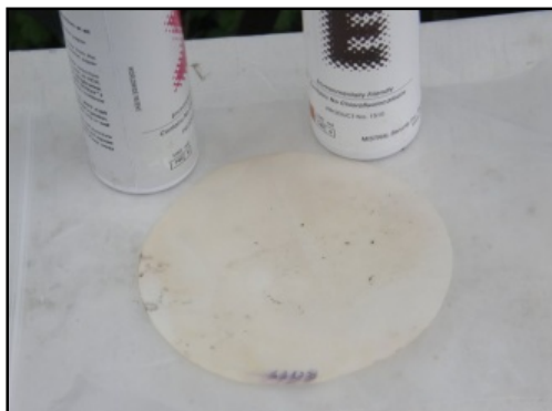
Figure A.2. Acetone was dripped onto one of the TS 50 mines and collected on this filter paper. No reaction is seen after both reagents were sprayed onto the paper. This result is typical of what was found for the other mines.
