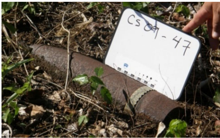
Figure C.6. 105-mm rounds sampled at Vieques with no HE found in soils.
