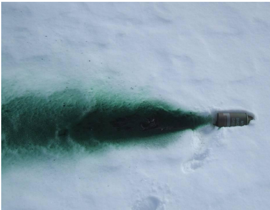
Figure 9. Residue on snow from detonation of M18 Green Signal Smoke Hand Grenade from sideways test.
