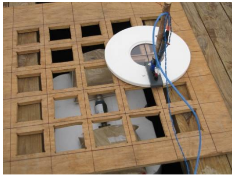
Figure 5-3 – The position template (left) over a test article and b) shown schematically (right).
