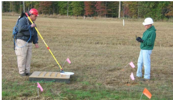
Figure 5-4 – The NRL TEMTADS Hand-Held Sensor
