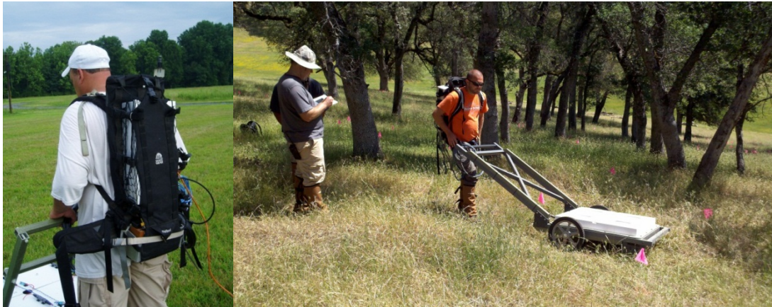
Figure 5-2 – TEMTADS 2x2 Electronics Backpack (left) TEMTADS MP 2x2 Cart and Data Acquisition Operators (right)
