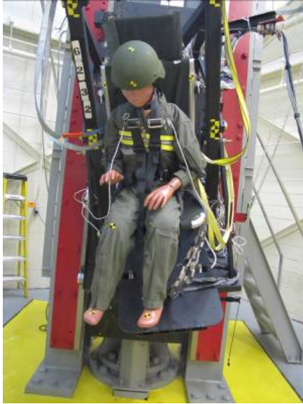
VDT6233 – Cell A, CV, H-60A/L aft-facing, LOIS, 23.23G, 38.56ft/s, 30.2ms rise time
