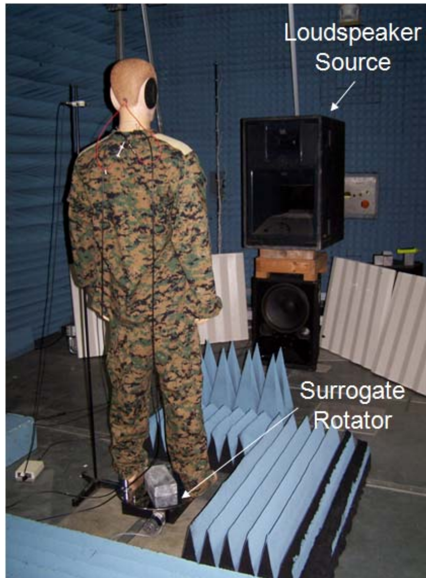
Fig. 2 — Laboratory experimental configuration. The surrogate is mounted on a rotator that allows for 360 degree aspect rotation relative to the acoustic source.
