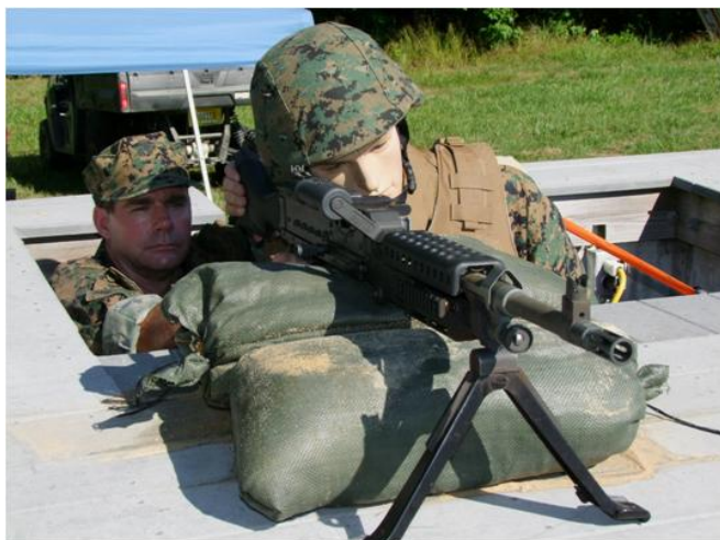
Fig. 9 — Human surrogate with helmet and armor positioned during foxhole firing measurements.
