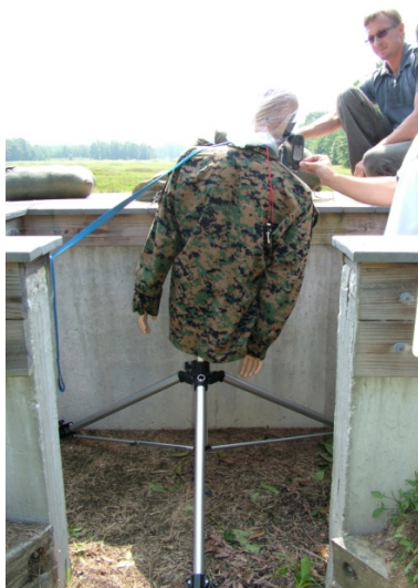
Fig. 10 — Tripod support for surrogate from the backside of foxhole
