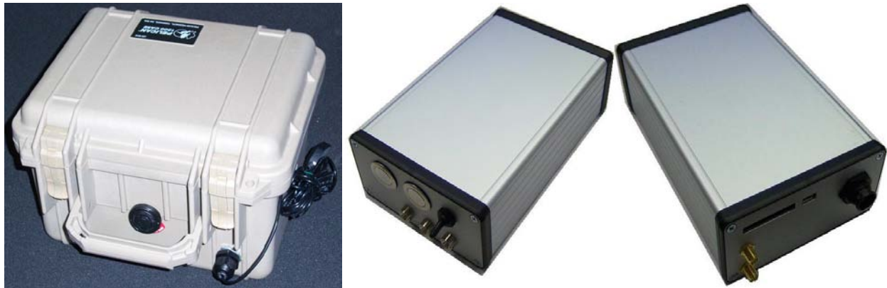
Figure 5. VDMTS Hardware. The photo on the left illustrates the hardware in the durable case The photos on the right illustrate the front and back panels of the VDMTS unit.
