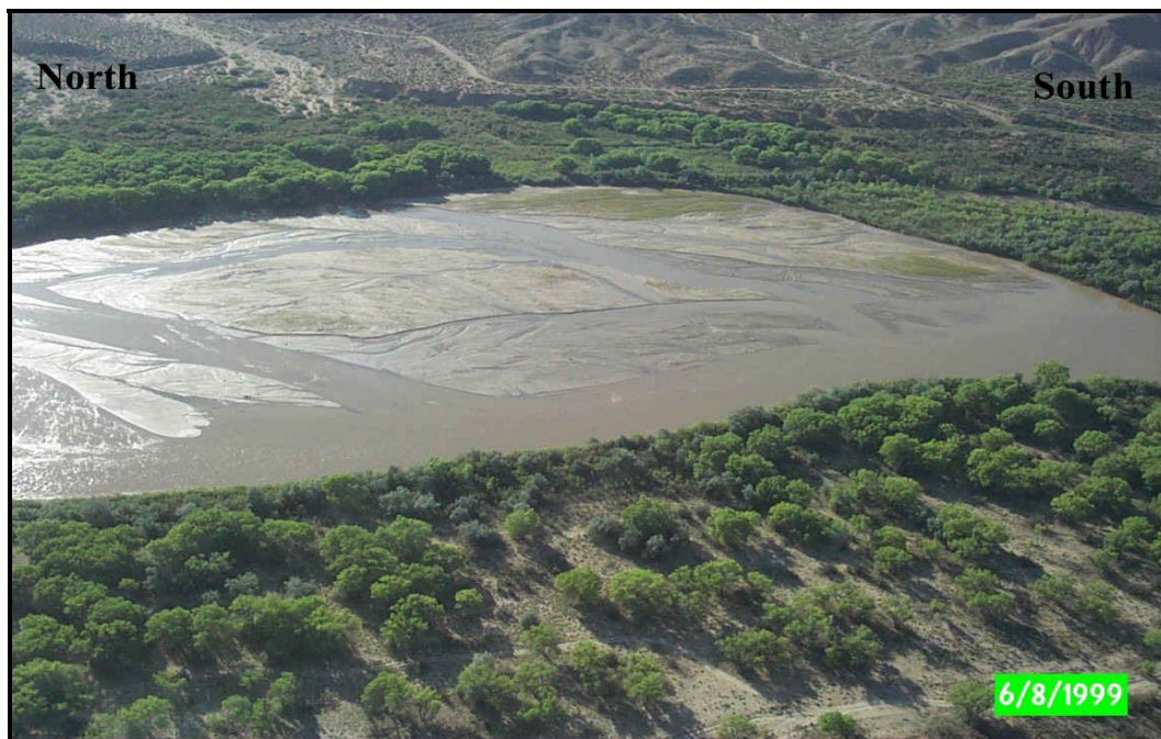
Figure 28. The middle Rio Grande is often characterized by numerous sandbars and a straight channel resulting from the placement of jetty jack fields and levees.
