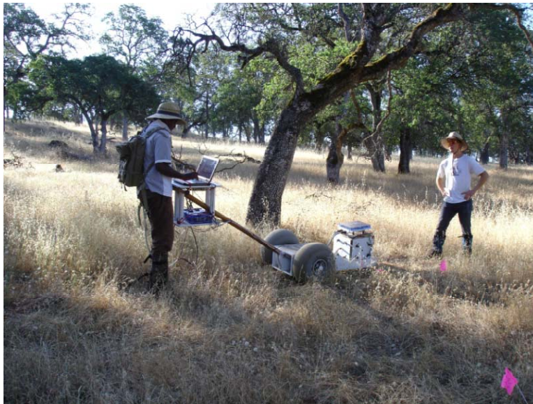
Figure 4-6. Portable Berkeley UXO Discriminator at Camp Beale
