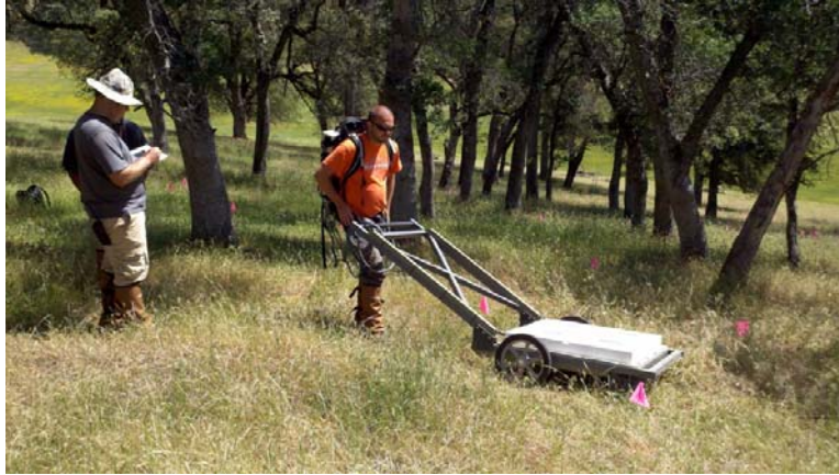
Figure 4-4. Portable TEMTADS 2x2 data acquisition at Beale
