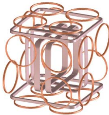
Figure 4-5. Transmit and receive coil configuration for the prototype portable UXO discriminator
