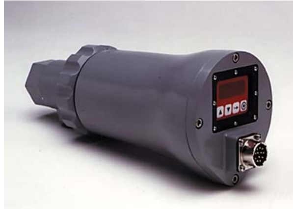
Figure 39 –Flame scanners verify the existence of a flame at the burner. They are interlocked with the fuel supply, representing an important safety component for every boiler.
