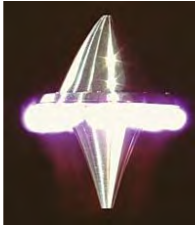
Figure 1.2. Original Type 100 lightcraft with laser induced air plasma.
