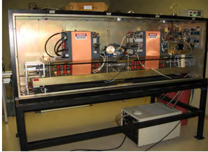
Figure D.1: Interior view of Lumonics K-922M TEA CO 2 laser module.
