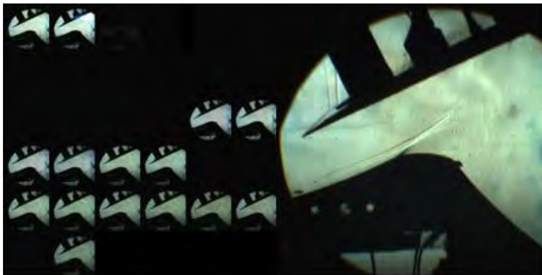
Figure 5.7: Left: Run #1—Erratic Schlieren image sequence . Note oversaturation of 2 nd frame when laser induced breakdown occurred, and missing frames due to EMI. Right: Run #2—Schlieren image with laser OFF, revealing flow structure at M=8.56.
