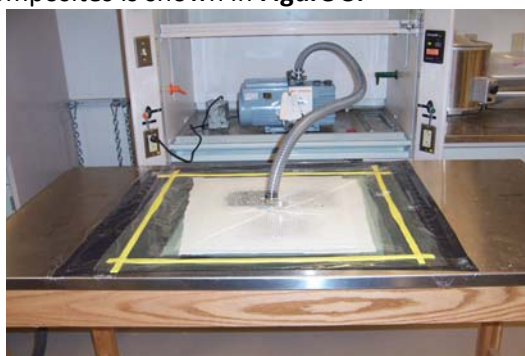
Figure 3: Fabrication of carbon fiber fabric using the vacuum assisted hand lay-up technique
