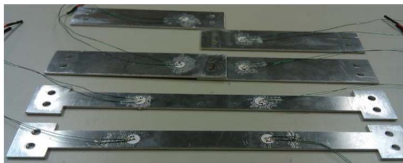
Figure 81 Lap bolted joint beams and beams carrying an adhesive test.
