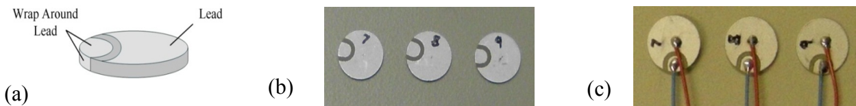
Figure 101 a) Circular PWAS diagram with wrap around electrode. b) Test samples for free-free test fixture. c) Test samples with soldered leads.
