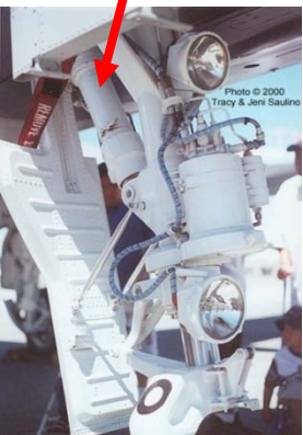
A-10 drag brace (300M - 270 ksi) Simple tension loading No forging required Corrosion related failures
