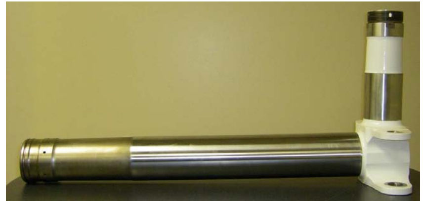
A-10 main landing gear piston (4330V – 240 ksi) More complex loading Forged component
