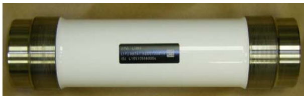
A-10 drag brace (300M - 270 ksi) Simple tension loading No forging required Corrosion related failures
